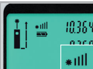
Assess reflection strength by means of scale reading
